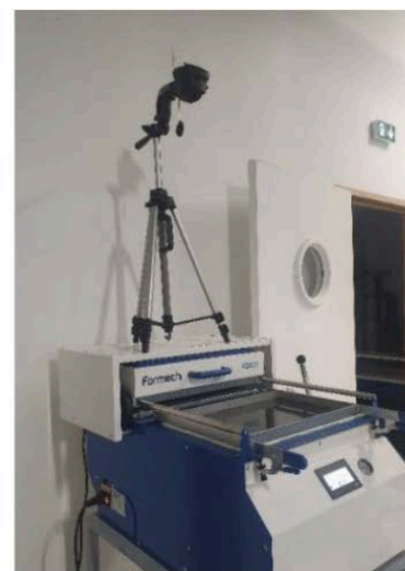
Fig. 9. Experimental thermoforming setup with Formech 450DT thermoforming machine and thermal camera.
