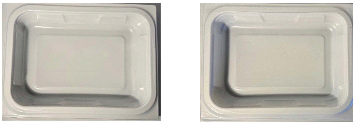
Figure 3: Food trays thermoformed from F_T1 sheet (left) and F_T2 sheet (right)
