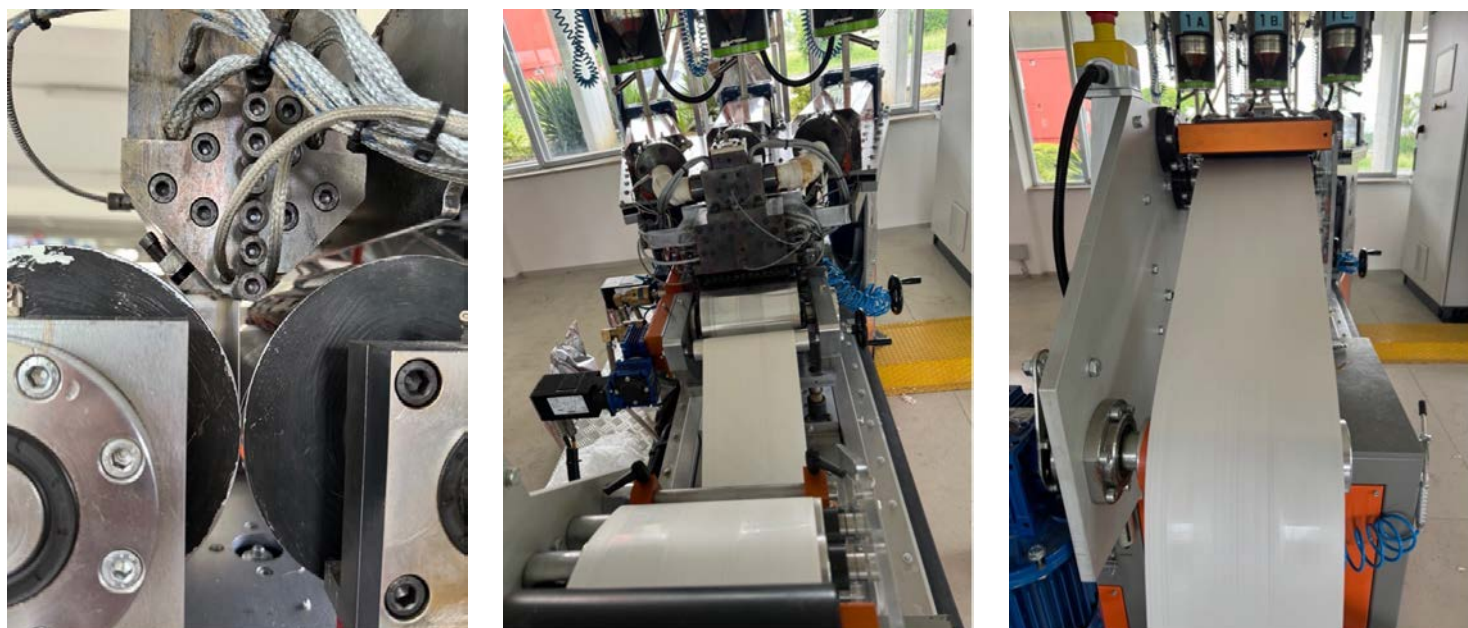
Figure 2: Cast extrusion process on EUR.EX.MA MiniCast Coex 5.
