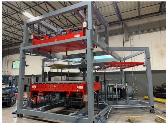
AVT Maac 5' x 8' Pressureformer
