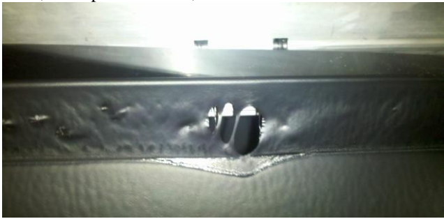
Figure 4 (Tears in back of formed sheet)
