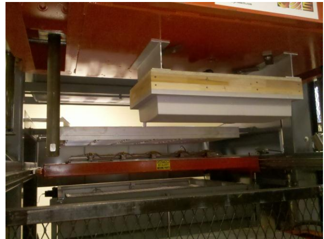
Figure 3 (Renshape mold on top platen)
